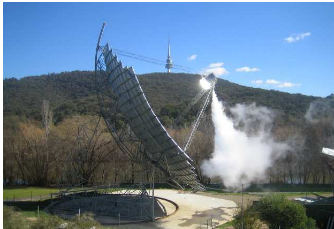
Fig. 1. An early test involving venting of steam from the SG4 receiver. Later tests have conveyed the steam to our 50 kWe steam turbine; the new dish is oversized for the current engine, so some venting is still required.
